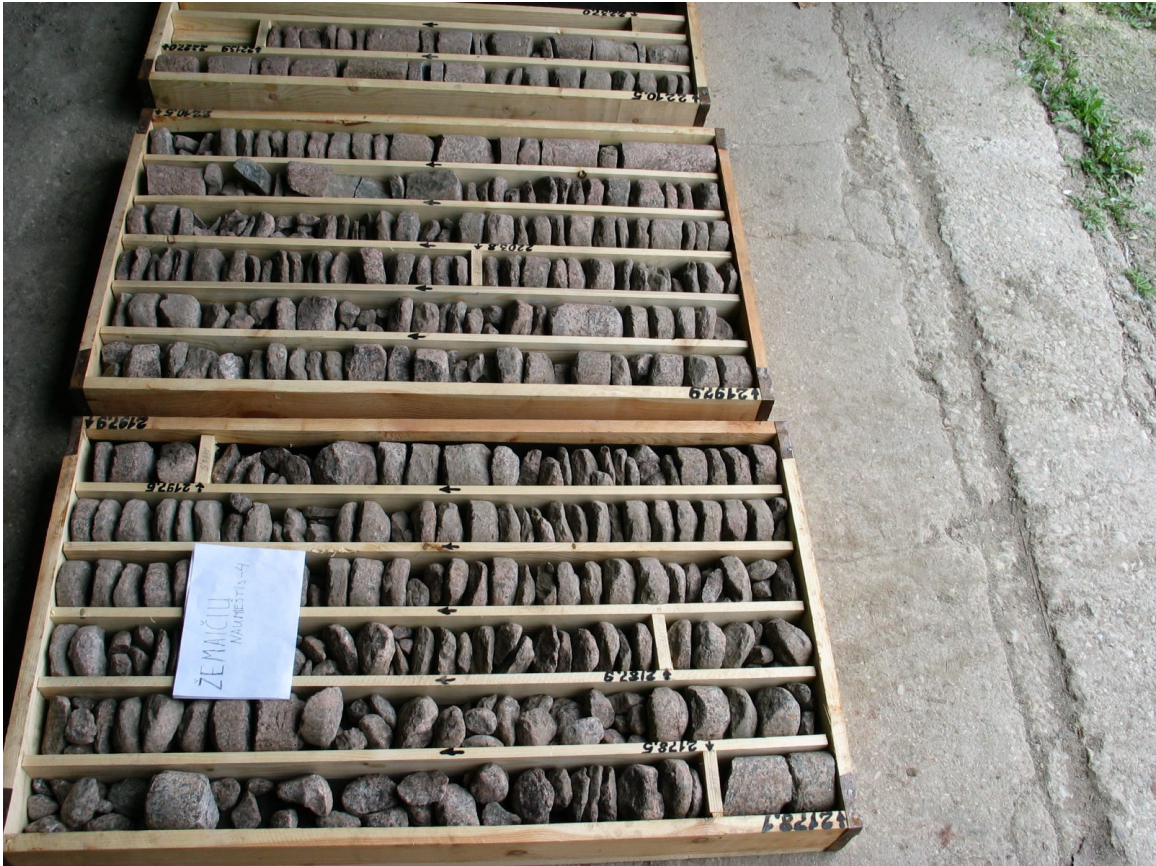
Fig.11. ZNI lithologies showing intense fracturing. The drilling discing is caused by abundant low-angle fractures. At the depth greater than 2008 m the fracturing decreases.
